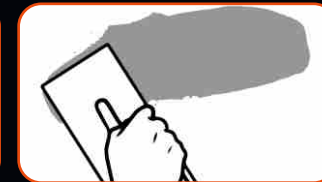
phase II: Apply the coloured Sandstone using a Venetian trowel.
