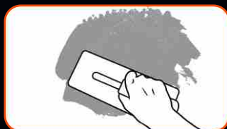
phase II: Apply coloured Sandstone with a venetian trowel.
